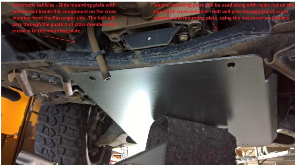
Automatic vehicles - Slide mounting plate with welded nut inside this component on the cross member from the Passenger side. The bolt will pass through the guard and cross member and screw in to the mounting plate.
